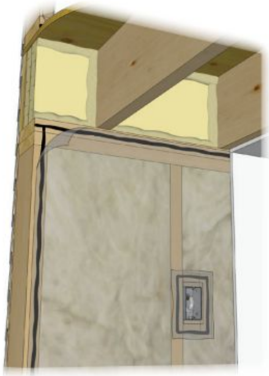
Sealed Polyethylene Approach
